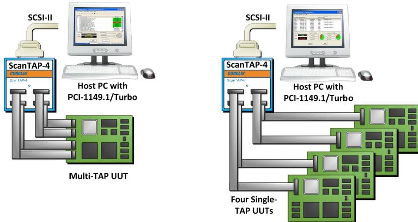
**PCI-1149.1/Turbo with ScanTAP-4 Configurations.**
