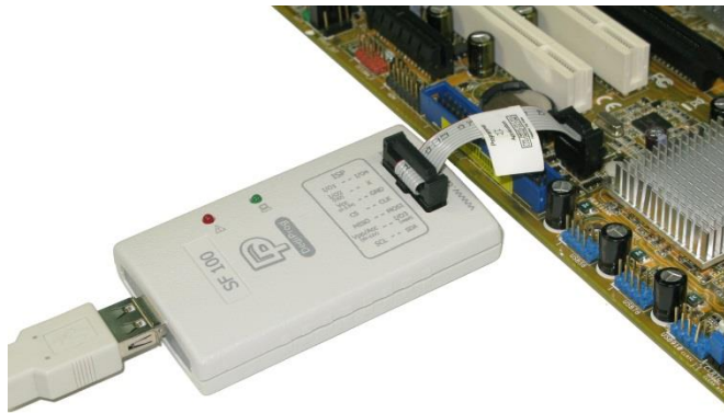
Fig 2: SF100 connected to the application pin header
