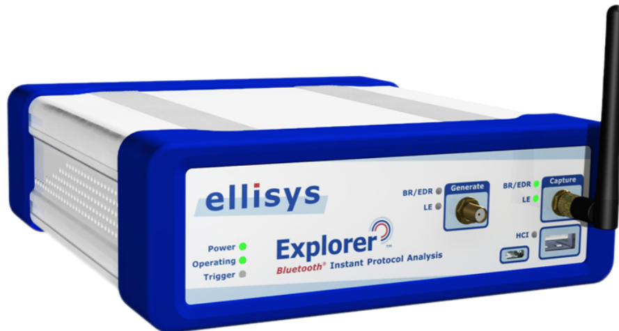
Figure 1-1 Bluetooth Explorer 400 (BEX400) All-in-One Protocol Analysis System
