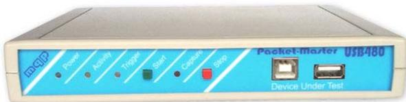
The USB480+ adds the capability of High Speed USB analysis. In addition a 64 MB FIFO prevents loss of data.
