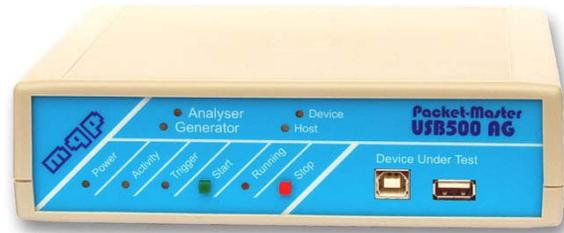
In addition to the capabilities of the USB480+, the USB500 AG analyser can also be configured as a USB generator. In host mode, it provides the  $V_{BUS}$  supply, applies bus states, and sends packets and waits for responses, all under control of your script.
