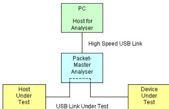
The Packet-Master USB12 will function correctly when connected to a Full Speed link but the capacity will be severely reduced and only low rates of USB traffic may be captured from the device under test.
