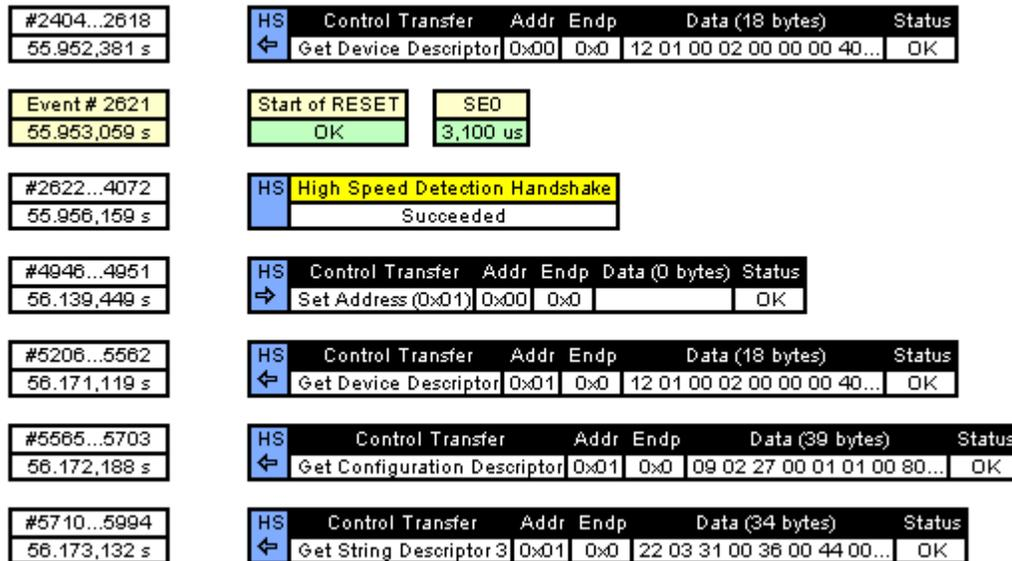
By clicking on the filter buttons for less significant events, the sequence of top-level control transfer header rows may be viewed in isolation. This ability to view information at an appropriate level of complexity makes GraphicUSB an invaluable tool for getting straight to the heart of the subject.
