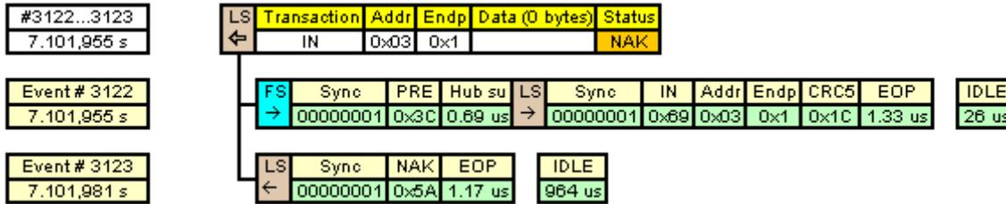
This view of part of a screen-shot from Graphic USB shows a representation of data being transferred at two different speeds on the same link. Each packet is preceded by a coloured marker indicating Full Speed or Low Speed. This makes the function of the PREAMBLE packet very clear. Each Event has a precise timestamp (left). Notice also the detailed timing information for Hub Setup time, End Of Packet duration, and IDLE state time.
