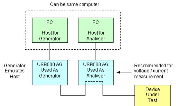
In this example a second USB500 AG is used as an analyser to capture the resulting traffic.
