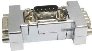
The IC57040-CAN-T is used to connect the IOM6 CAN/LIN Accessory to a CAN bus by splitting the existing bus connection – position F on the diagram below. The existing CAN bus connection is split using the IC57040-CAN-T allowing the IOM6 CAN/LIN Accessory to connect to it using an IC57040-CAN-DB9 cable (no termination required).
