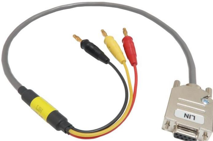
The IC57040-LIN-JACK cable is used to connect the IOM6 CAN/LIN Accessory to an existing LIN network via banana jack connectors. The cable length is 0.65m. The cable connects to the LIN1 or LIN2 connector.
