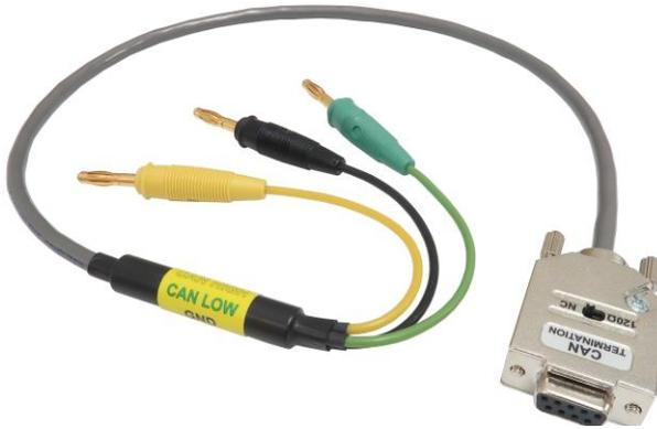
The IC57040-CAN-DB9 is used to connect the IOM6 CAN/LIN Accessory to an existing CAN network through the banana jacks. The 120 Ohm termination impedance is selected using the switch located on the cable DB9 connector. Cable length is 0.65m.
